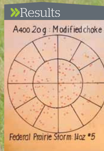
BELOW This ammunition gave dense Full choke patterns from the Modified tube.
