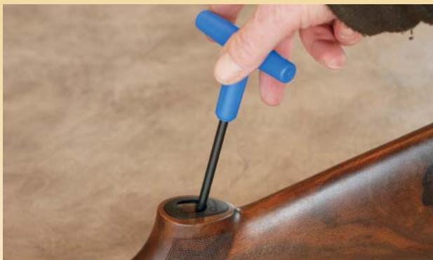
Top; The action exposed. If needed, the trigger group can also be removed simply, using the stock bolt Torx key. Above: The Kick-Off system makes for soft shooting. Left: Q-stock enables the stock to be removed quickly through the pistol grip cap.
